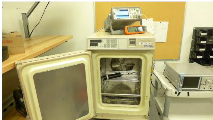
Figure D-1 - Test Setup for Frequency Stability
