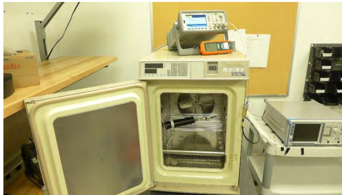
Figure D-1 - Test Setup for Frequency Stability
