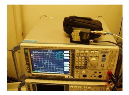
Figure C-1. Test Setup for Necessary Bandwidth Tests
