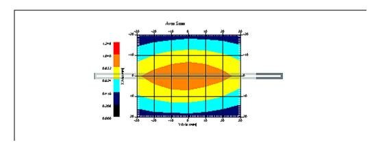
1 gram SAR value : 0.951 W/kg 10 gram SAR value : 0.623 W/kg Area Scan Peak SAR: 1.042 W/kg Zoom Scan Peak SAR : 1.461 W/kg
