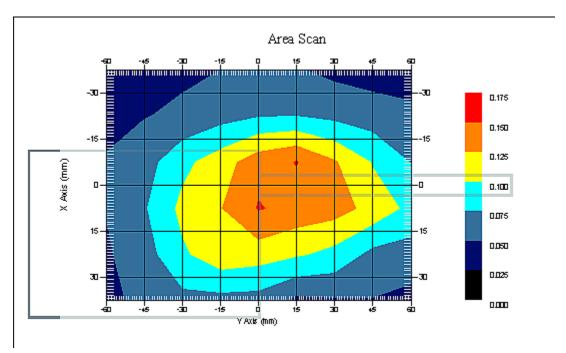
1 gram SAR value : 0.154 W/kg 10 gram SAR value : 0.113 W/kg Area Scan Peak SAR : 0.152 W/kg Zoom Scan Peak SAR : 0.200 W/kg
