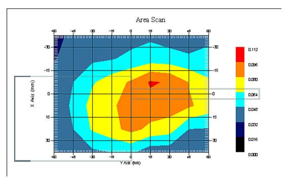
1 gram SAR value : 0.110 W/kg 10 gram SAR value : 0.099 W/kg Area Scan Peak SAR : 0.098 W/kg Zoom Scan Peak SAR : 0.130 W/kg
