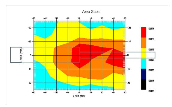
1 gram SAR value : 0.082 W/kg 10 gram SAR value : 0.064 W/kg Area Scan Peak SAR : 0.083 W/kg Zoom Scan Peak SAR : 0.120 W/kg
