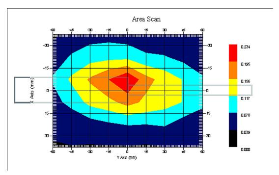
1 gram SAR value : 0.215 W/kg 10 gram SAR value : 0.137 W/kg Area Scan Peak SAR : 0.234 W/kg Zoom Scan Peak SAR : 0.330 W/kg
