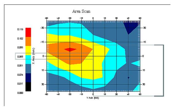
1 gram SAR value : 0.102 W/kg 10 gram SAR value : 0.079 W/kg Area Scan Peak SAR : 0.105 W/kg Zoom Scan Peak SAR : 0.130 W/kg
