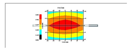
1 gram SAR value : 0.222 W/kg 10 gram SAR value : 0.195 W/kg Area Scan Peak SAR : 0.343 W/kg Zoom Scan Peak SAR : 0.512 W/kg
