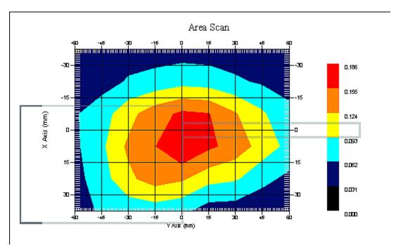
1 gram SAR value : 0.182 W/kg 10 gram SAR value : 0.130 W/kg Area Scan Peak SAR : 0.186 W/kg Zoom Scan Peak SAR : 0.270 W/kg
