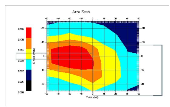
1 gram SAR value : 0.163 W/kg 10 gram SAR value : 0.115 W/kg Area Scan Peak SAR : 0.155 W/kg Zoom Scan Peak SAR : 0.210 W/kg
