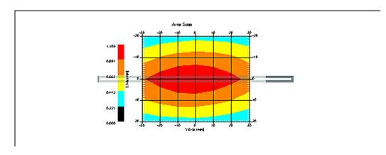
1 gram SAR value : 0.889 W/kg 10 gram SAR value : 0.574 W/kg Area Scan Peak SAR : 1.112 W/kg Zoom Scan Peak SAR : 1.568 W/kg
