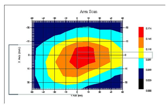
1 gram SAR value : 0.165 W/kg 10 gram SAR value : 0.119 W/kg Area Scan Peak SAR : 0.171 W/kg Zoom Scan Peak SAR : 0.230 W/kg
