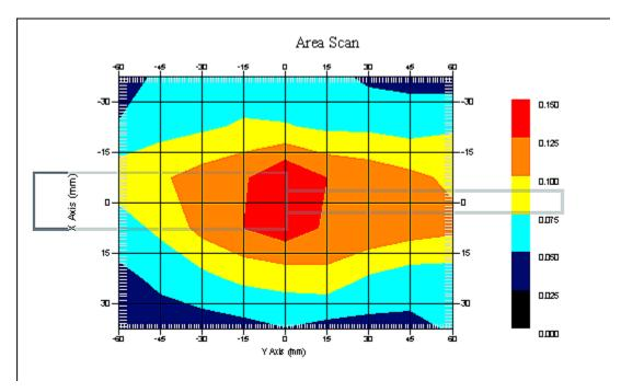
1 gram SAR value : 0.160 W/kg 10 gram SAR value : 0.110 W/kg Area Scan Peak SAR : 0.149 W/kg Zoom Scan Peak SAR : 0.230 W/kg
