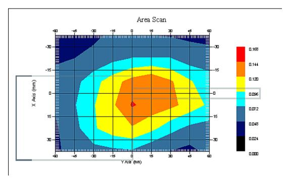
1 gram SAR value : 0.144 W/kg 10 gram SAR value : 0.112 W/kg Area Scan Peak SAR : 0.147 W/kg Zoom Scan Peak SAR : 0.170 W/kg
