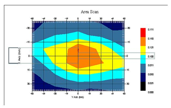
1 gram SAR value : 0.162 W/kg 10 gram SAR value : 0.115 W/kg Area Scan Peak SAR : 0.151 W/kg Zoom Scan Peak SAR : 0.230 W/kg
