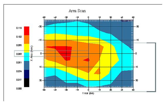
1 gram SAR value : 0.115 W/kg 10 gram SAR value : 0.087 W/kg Area Scan Peak SAR : 0.104 W/kg Zoom Scan Peak SAR : 0.150 W/kg
