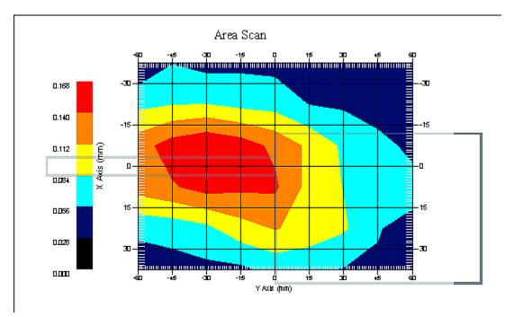
1 gram SAR value : 0.171 W/kg 10 gram SAR value : 0.121 W/kg Area Scan Peak SAR : 0.167 W/kg Zoom Scan Peak SAR : 0.230 W/kg
