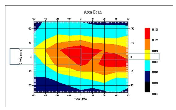
1 gram SAR value : 0.130 W/kg 10 gram SAR value : 0.089 W/kg Area Scan Peak SAR : 0.125 W/kg Zoom Scan Peak SAR : 0.190 W/kg
