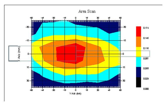
1 gram SAR value : 0.191 W/kg 10 gram SAR value : 0.125 W/kg Area Scan Peak SAR : 0.174 W/kg Zoom Scan Peak SAR : 0.300 W/kg
