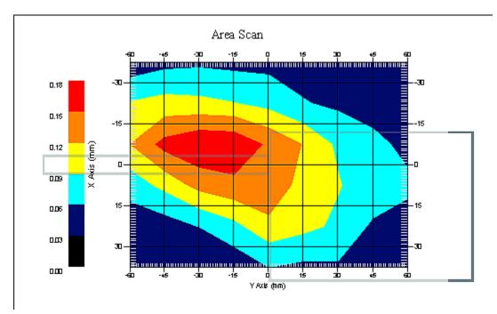
1 gram SAR value : 0.155 W/kg 10 gram SAR value : 0.110 W/kg Area Scan Peak SAR : 0.179 W/kg Zoom Scan Peak SAR : 0.230 W/kg
