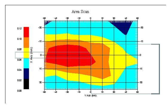
1 gram SAR value : 0.127 W/kg 10 gram SAR value : 0.096 W/kg Area Scan Peak SAR : 0.118 W/kg Zoom Scan Peak SAR : 0.180 W/kg
