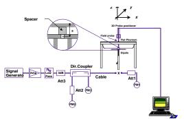
Figure 9.1 Dipole Validation Test Setup
