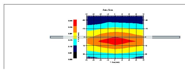
1 gram SAR value : 0.479 W/kg 10 gram SAR value : 0.322 W/kg Area Scan Peak SAR : 0.537 W/kg Zoom Scan Peak SAR : 0.796 W/kg
