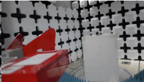
Figure 2: ULXD1 Transmitter Test Setup
