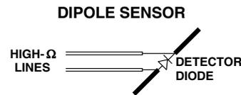
The SAR is assessed with the probe which moves at a default height of 5mm from the center of the diode, which is mounted to the sensor, to the phantom surface (Z height). The diagram above right shows how the center of the sensor is defined with the location of the diode placed at the center of the dipole. The 5mm default in the Z axis is the optimum height for assessing SAR where the boundary effect is at its least, with the probe located closest to the phantom surface (boundary).
