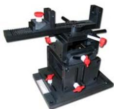
In combination with the SAM phantom, the mounting device enables the rotation of the mounted transmitter in spherical coordinates whereby the rotation point is the ear opening. The devices can easily, accurately, and repeatably be positioned according to the FCC specifications. The device holder can be locked at different phantom locations (left head, right head, and uni-phantom).
