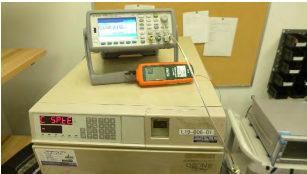
Figures D-1 - Test Setup for Frequency Stability
