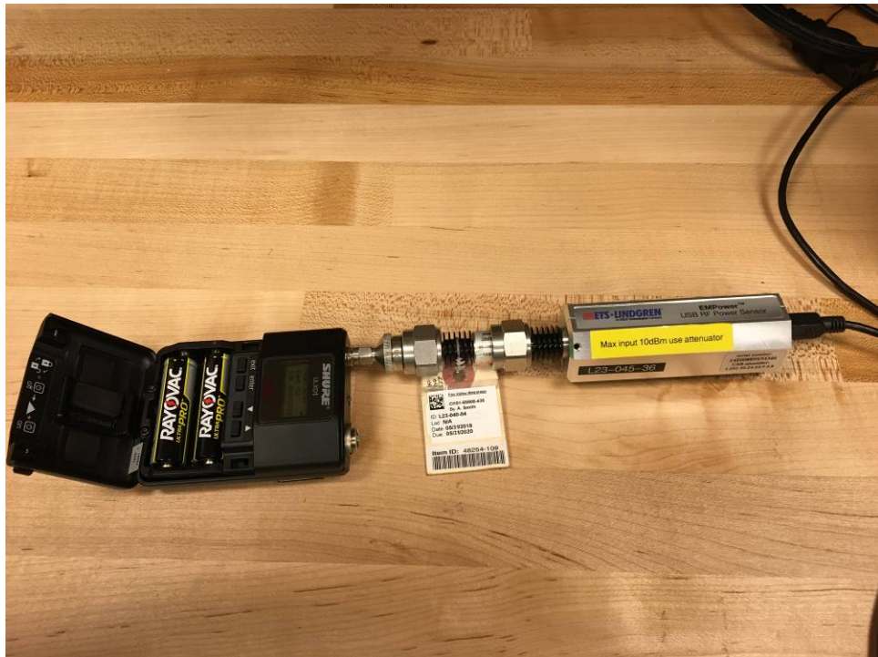
Test setup for maximum conducted output
