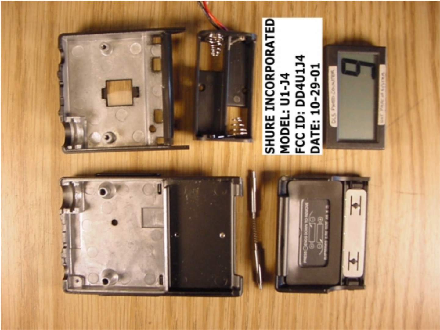
Battery Holder Removed/Inside Covers
