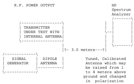
Equipment placed 1 meter above ground on a rotatable platform. The center of the Dipole antenna at the center of the platform and the output of the signal generator adjusted to produce the same meter reading as measured for the fundamental in the radiated emissions test.
