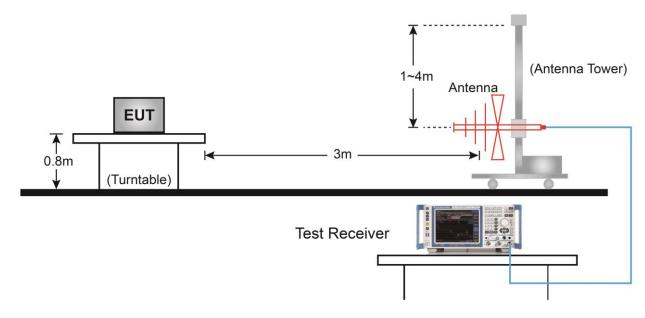
Above 1GHz Test Setup:
