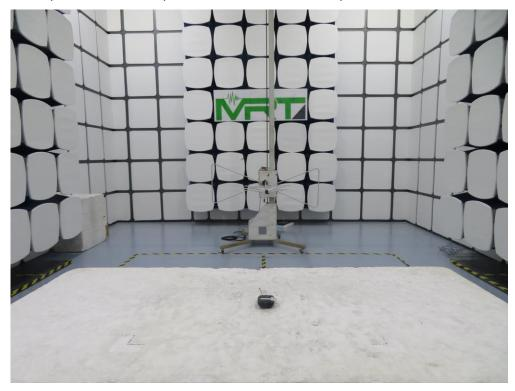
Description: Radiated Spurious Emission Test Setup for  $1GHz \sim 18GHz$
