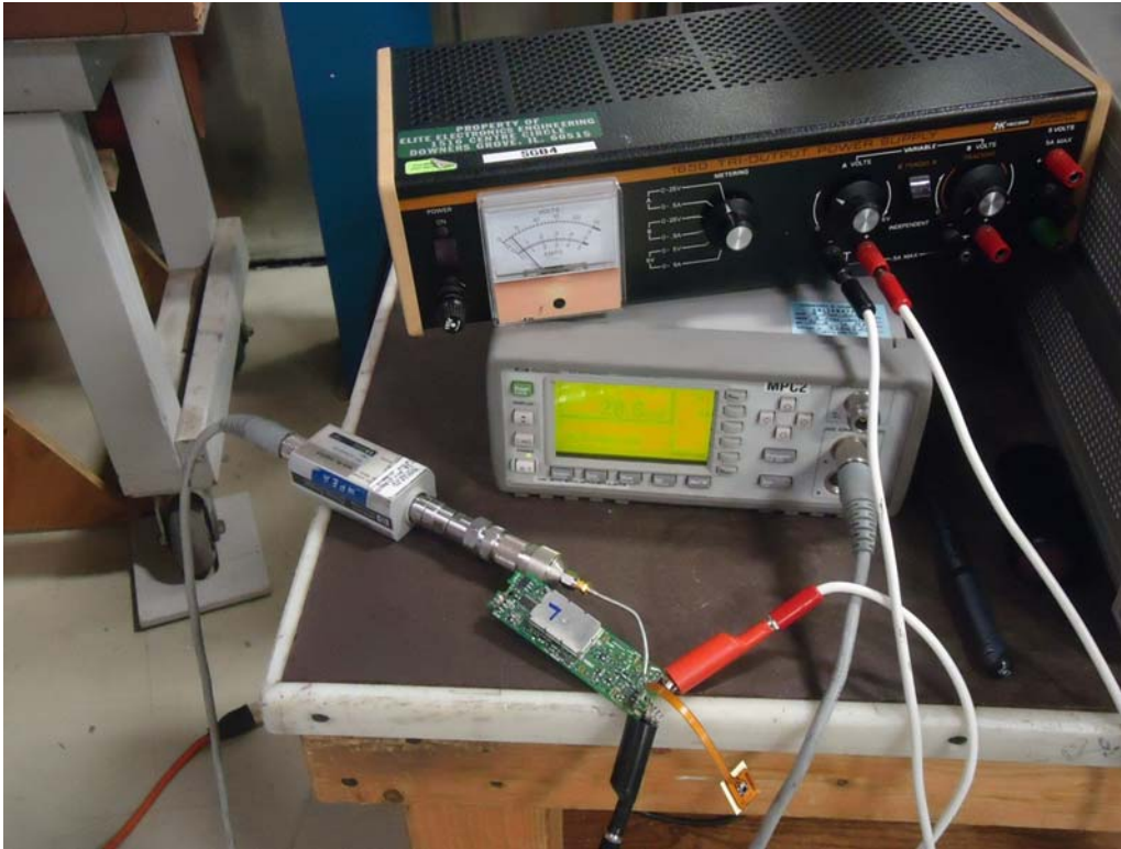
Test Setup for RF Output Power Test
