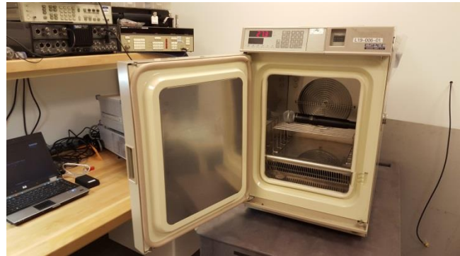
Figure B-2. Sample unit in temperature chamber
