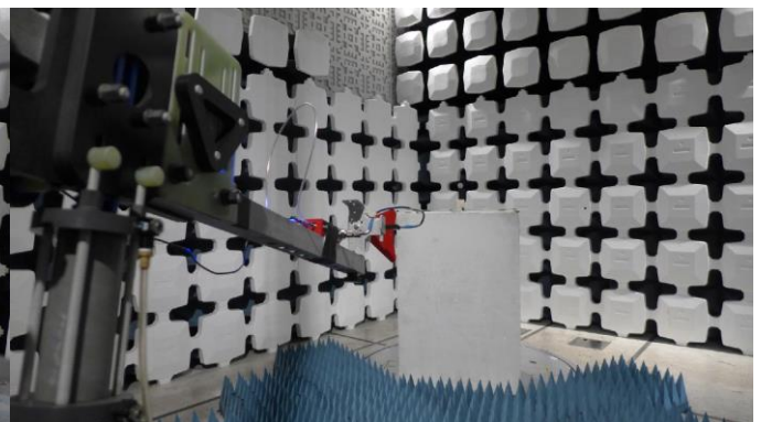
Figure 2: QLXD2 Transmitter Test Setup
