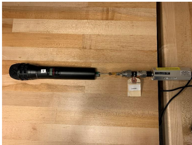
Figure C 1: Test setup for Maximum Power Output
