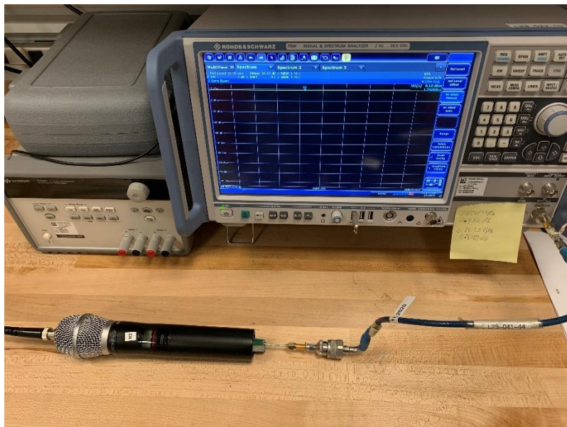
Figure A-1 - Test Setup for Necessary Bandwidth
