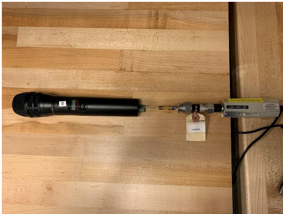
Figure C-1 – Maximum Radiated RF Output Power setup
