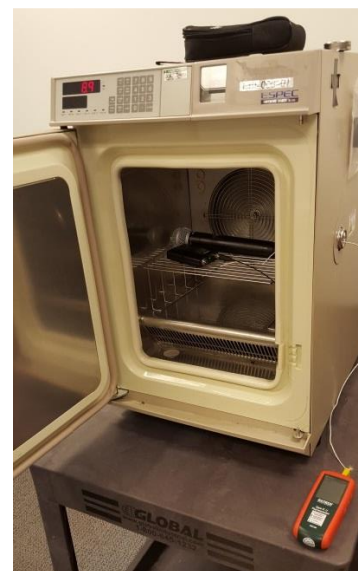
Figure B-2. Samples in Temperature Chamber
