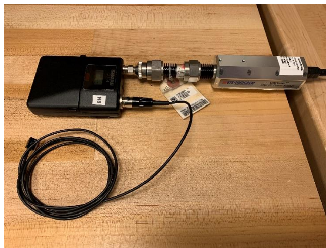
Figure C 1: Test setup for Maximum Power Output
