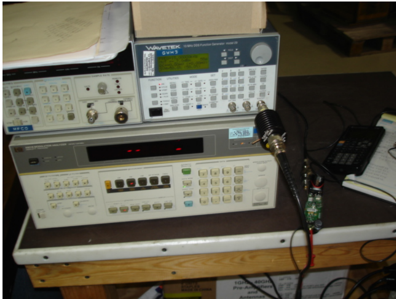
Output Power Test Set-up
