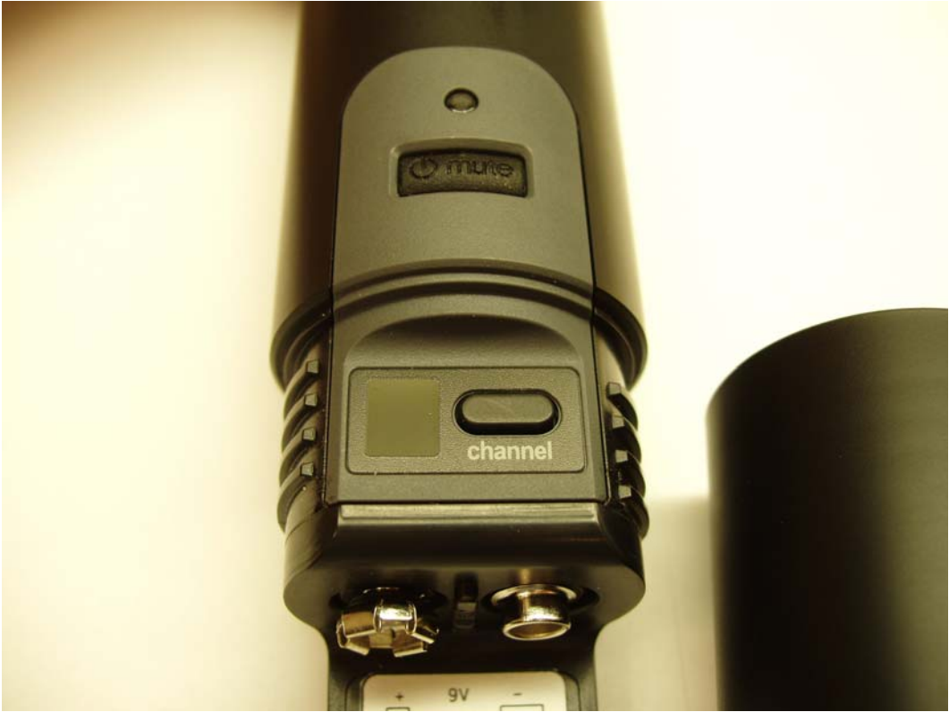
PG2 Control Switch
