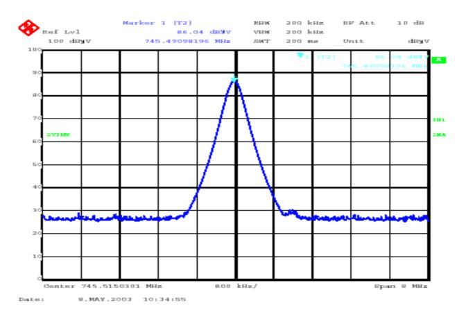
Output Power = 86.04 dBµV + 1.0 dB cable loss + 40.10 external atten. = 127.1 dBµV = 102.5 mW
