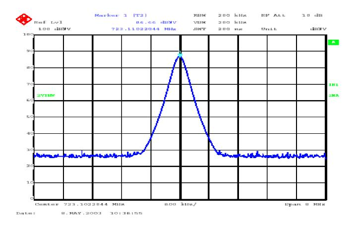
Output Power = 86.66 dBµV + 1.0 dB cable loss + 40.11 external atten. = 127.77 dBµV = 119.7 mW
