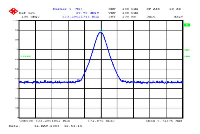
Output Power = 87.75 dBµV + 1.0 dB cable loss + 40.10 external atten. = 128.85 dBµV = 153.4 mW
