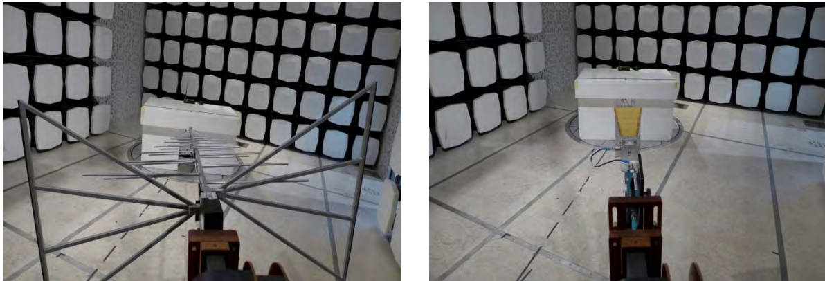
Figure H.5. Test Setup for Spurious Emissions 30MHz to 1GHz and 1GHz to 7GHz
