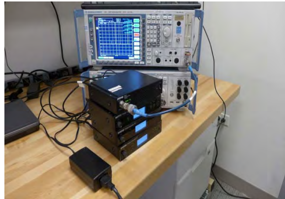
Figure H.3. Setup of Frequency Stability Measurement
