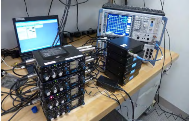
Figure H.7. Setup of Spurious Emissions at Antenna Terminals Measurement
