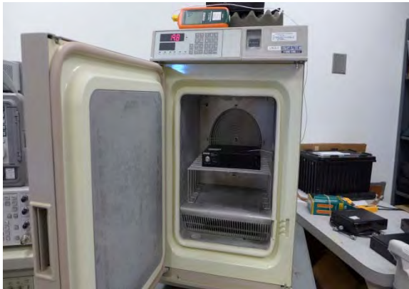
Figure H.3. Setup of Frequency Stability Measurement
