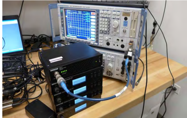
Figure H.7. Setup of Spurious Emissions at Antenna Terminals Measurement
