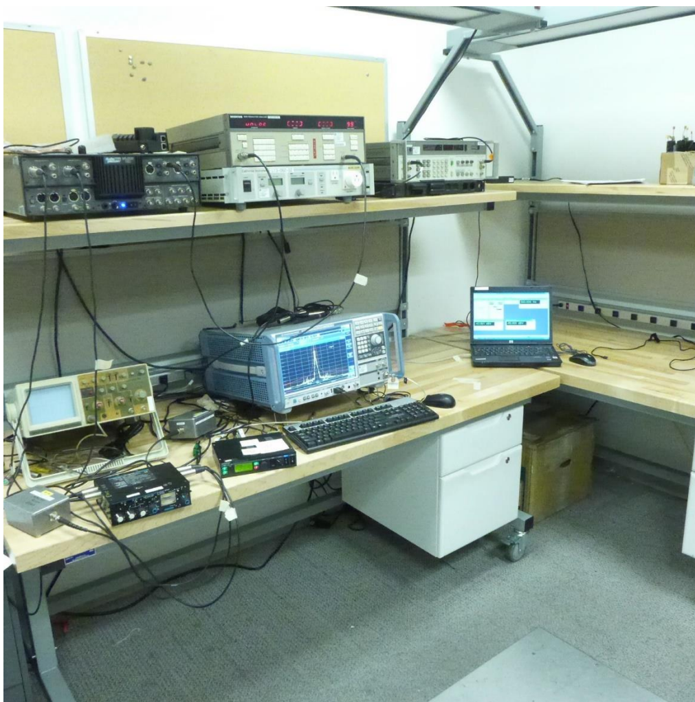
Figure A-1 - Test Setup for Necessary Bandwidth
