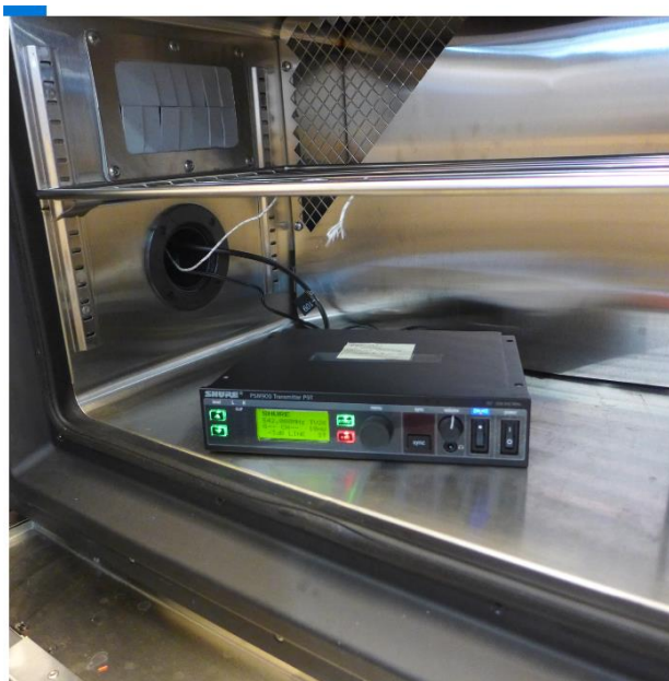
Figures D-1 - Test Setup for Frequency Stability
