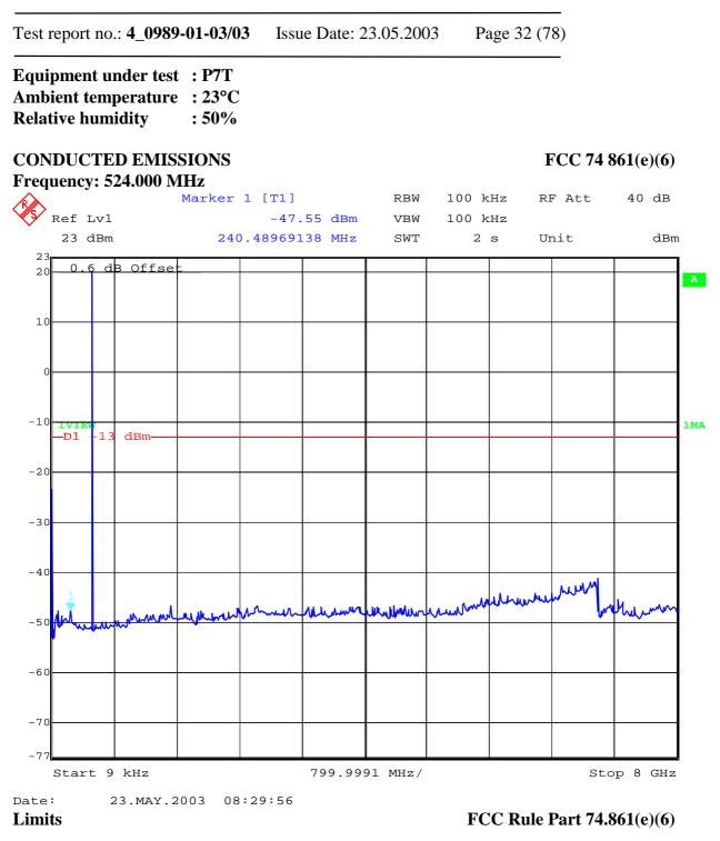
(6) The mean power of emissions shall be attenuated below the mean output power of the transmitter in accordance with the following schedule:
