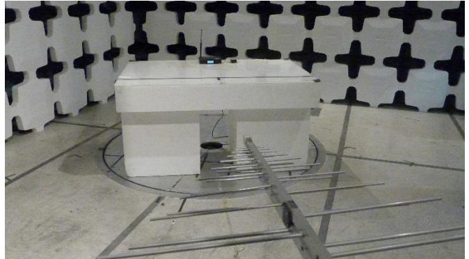
Figure D-1 - Test Setup for Spurious Emissions 30MHz to 1GHz
