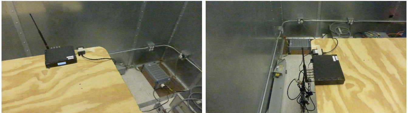
Figure E-1 - Test Setup for Conducted Emissions 150kHz to 30MHz
