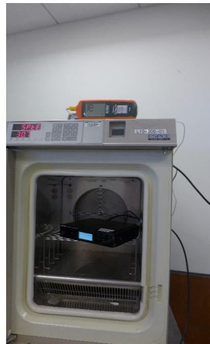
Figure B-1 - Test Setup for Frequency Stability
