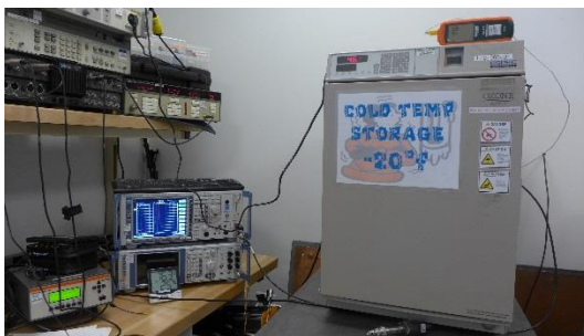
Figure B-1 - Test Setup for Frequency Stability
