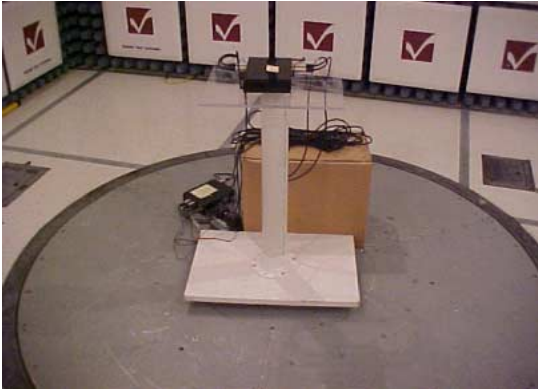
View of one of the PSM200 samples, while performing Radiated Emission Testing
