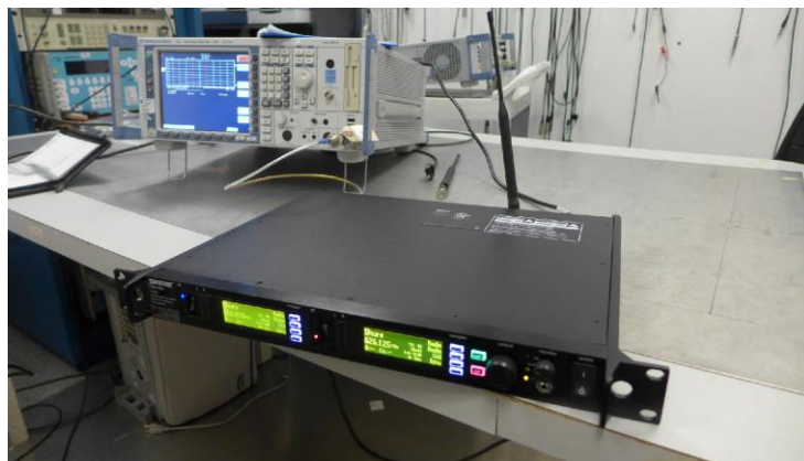
Figure 1: Test setup for Maximum Radiated Output
