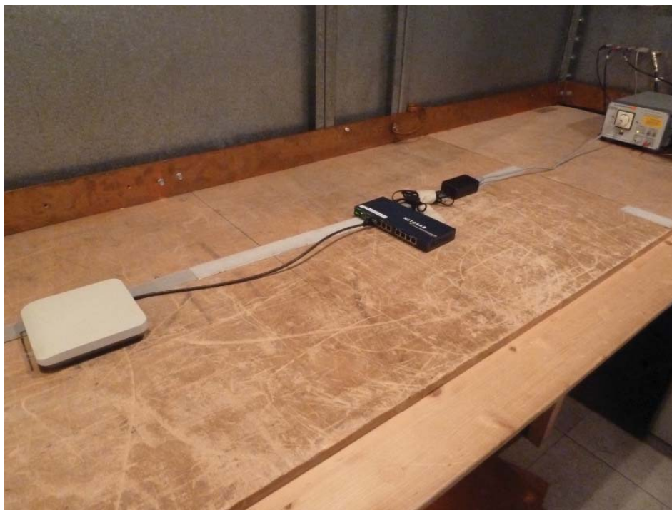
Photo 2: Power Line Conducted Emission Test
