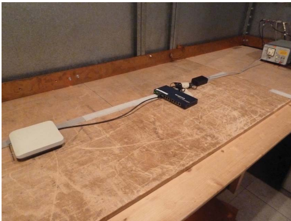
Photo 2: Power Line Conducted Emission Test
