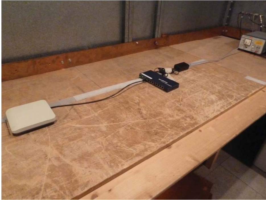
Photo 1: Power Line Conducted Emission Test
