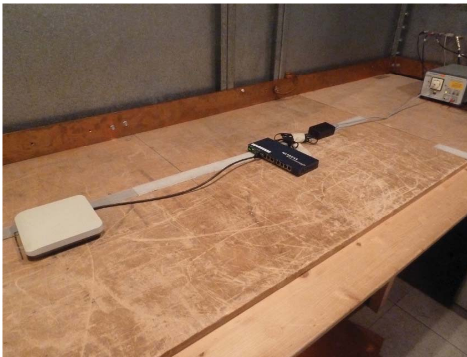
Photo 2: Power Line Conducted Emission Test
