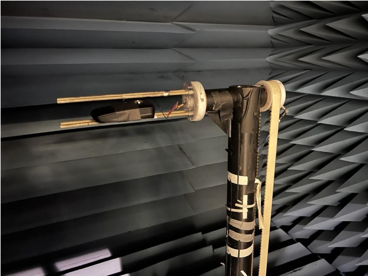
Figure 1-4. Photo of MXW8X in antenna test chamber.
