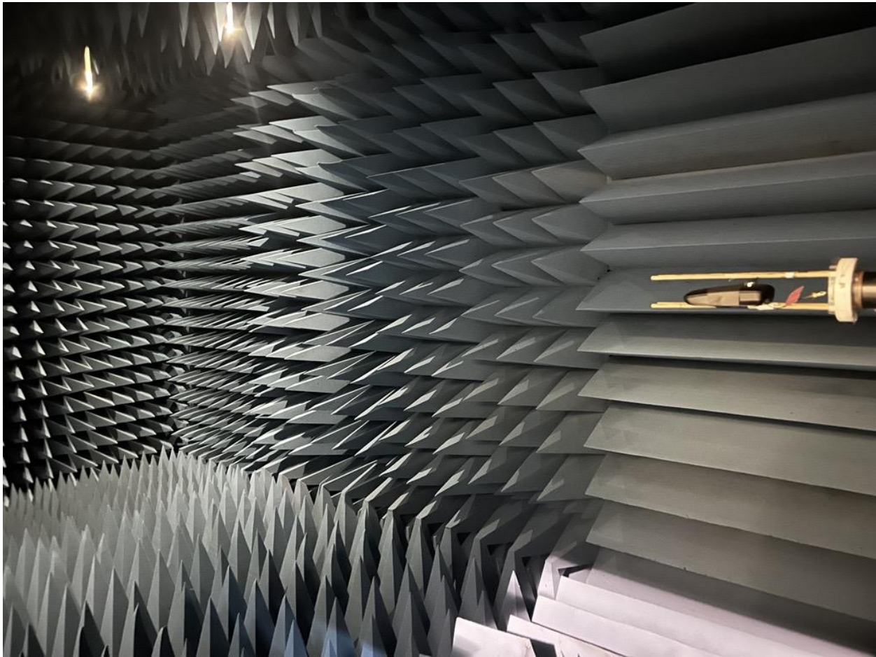
Figure 1-5. Photo of Shure's antenna test chamber with MXW8X ready for testing.
