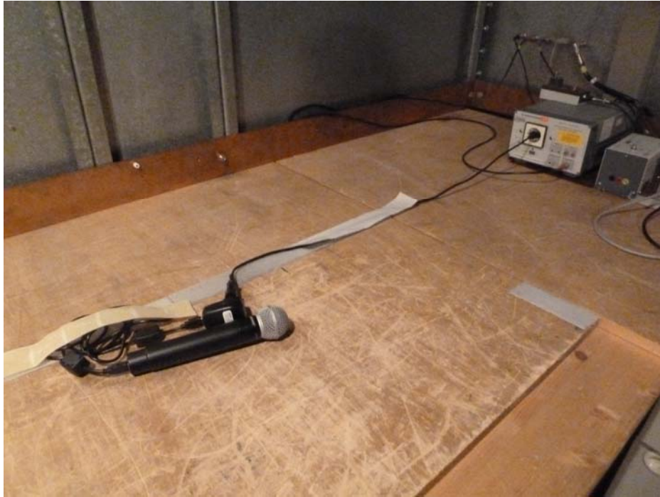
Photo 1: Power Line Conducted Emission Test
