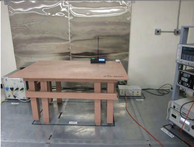
AC Conducted Emissions – Front View
