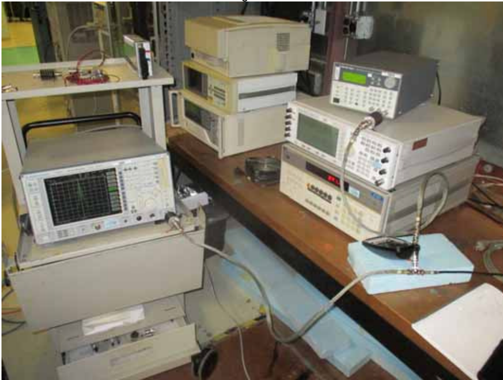
Test Setup for Occupied Bandwidth Test
