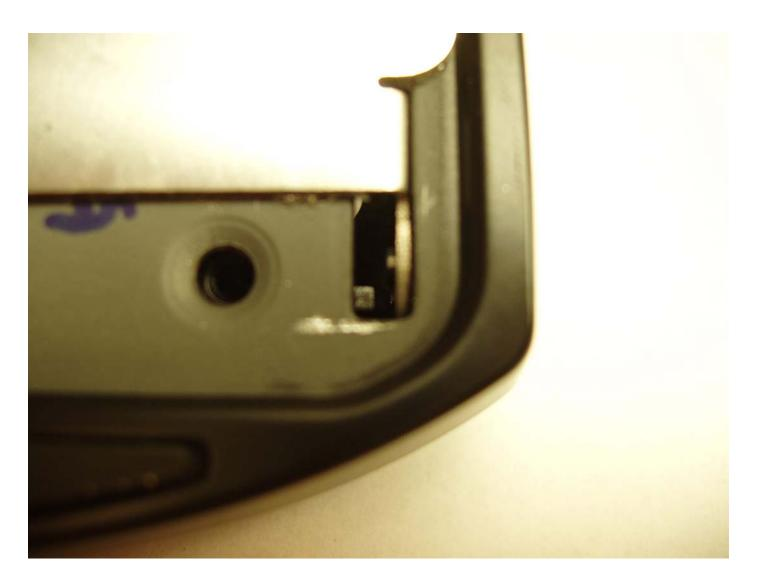
The wedge on the far right side that is used to prevent a screwdriver from removing the battery compartment door.
