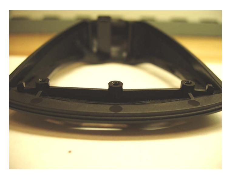
The wedge on the far left and right sides are used to prevent battery compartment door removal.
