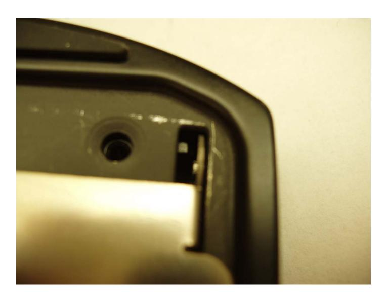
Another view showing the wedge that is used to prevent a screwdriver from removing the battery compartment door.
