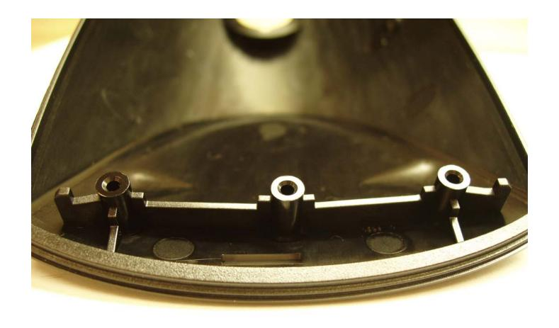
The wedge on the far left and right sides are used to prevent battery compartment door removal.
