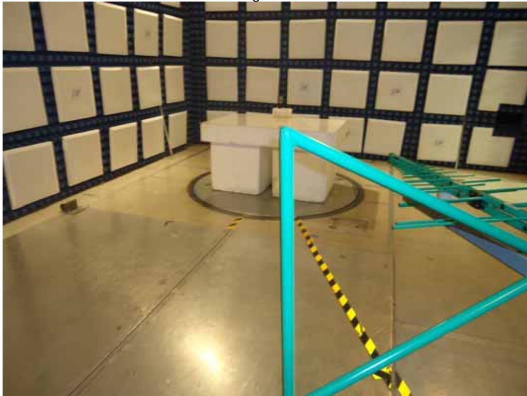
Test Setup for Radiated Emissions – 30MHz to 2GHz, Horizontal Polarization
