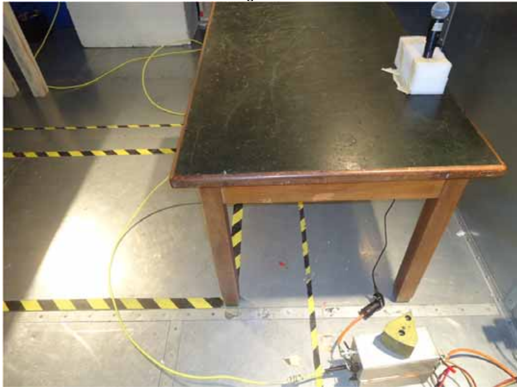
Test Setup for Conducted Emissions
