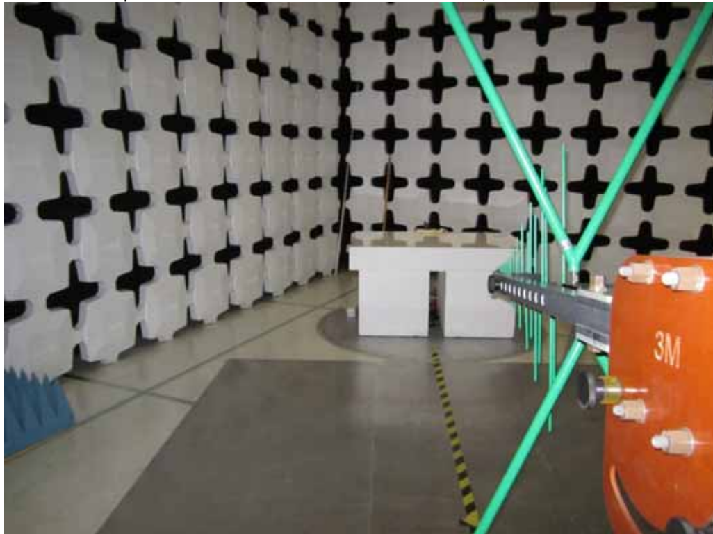
Test Setup for Radiated Emissions – 30MHz to 2GHz, Vertical Polarization
