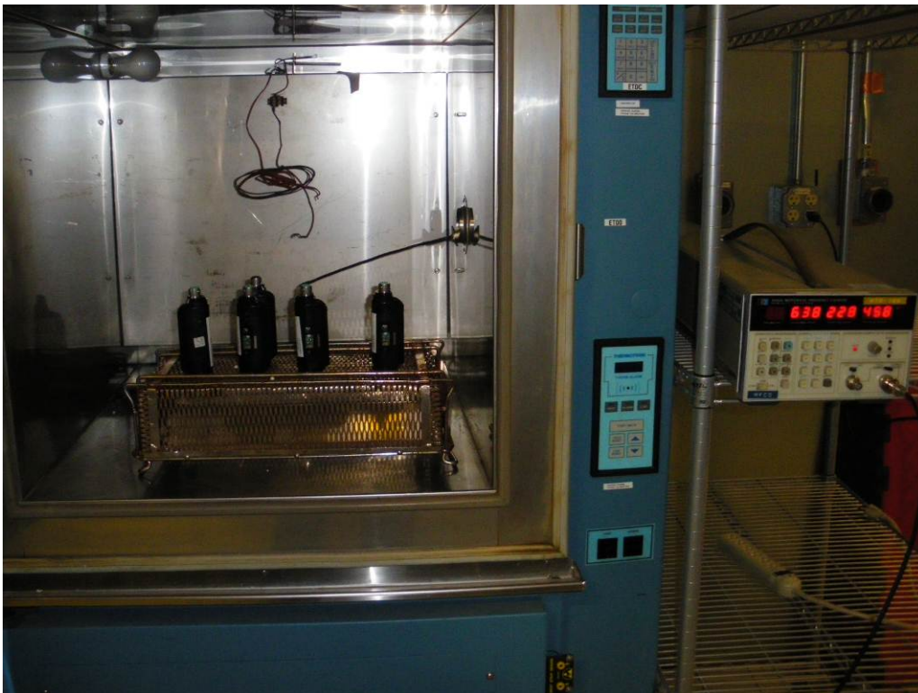
Test Setup for Frequency Stability over Temperature Test
