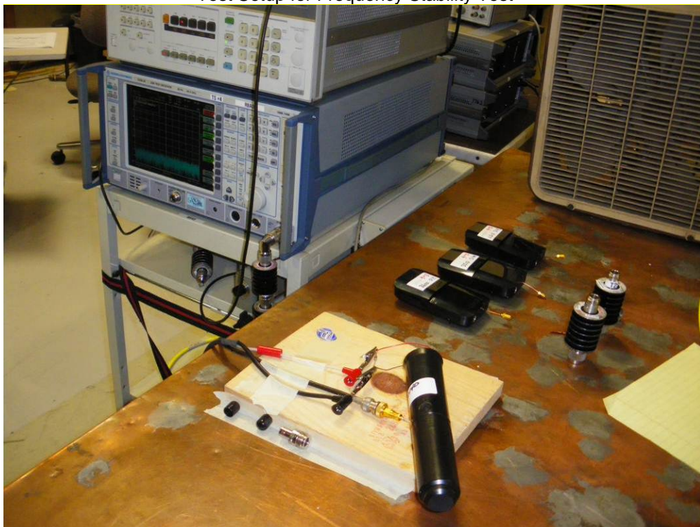
Test Setup for Occupied Bandwidth Test
