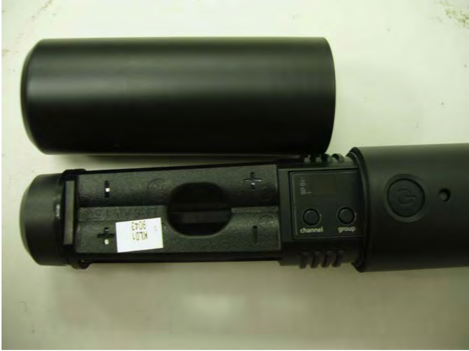
Shure BLX2 Front View – Battery Door Open
