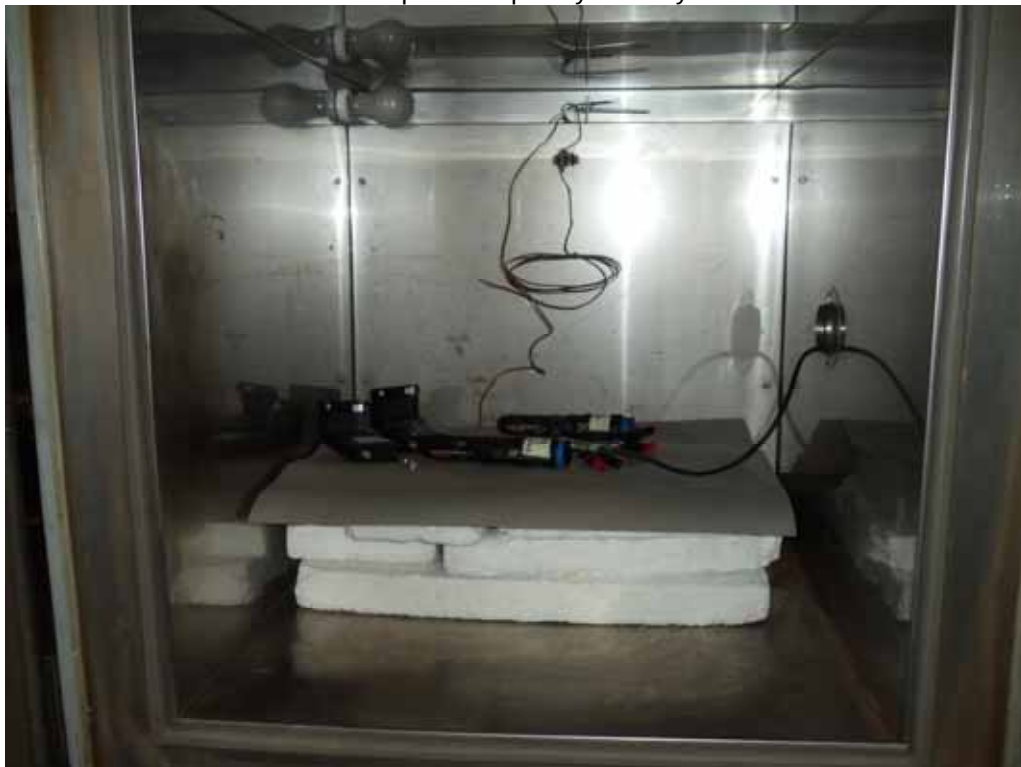
Test Setup for Occupied Bandwidth Test
