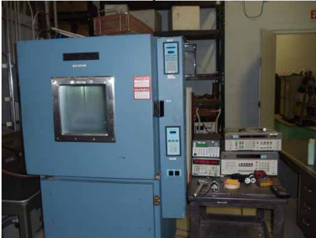
Test Setup for Frequency Stability Test
