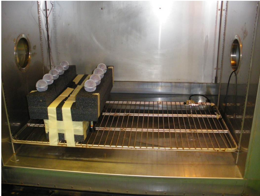
Test Setup for Frequency Stability Test
