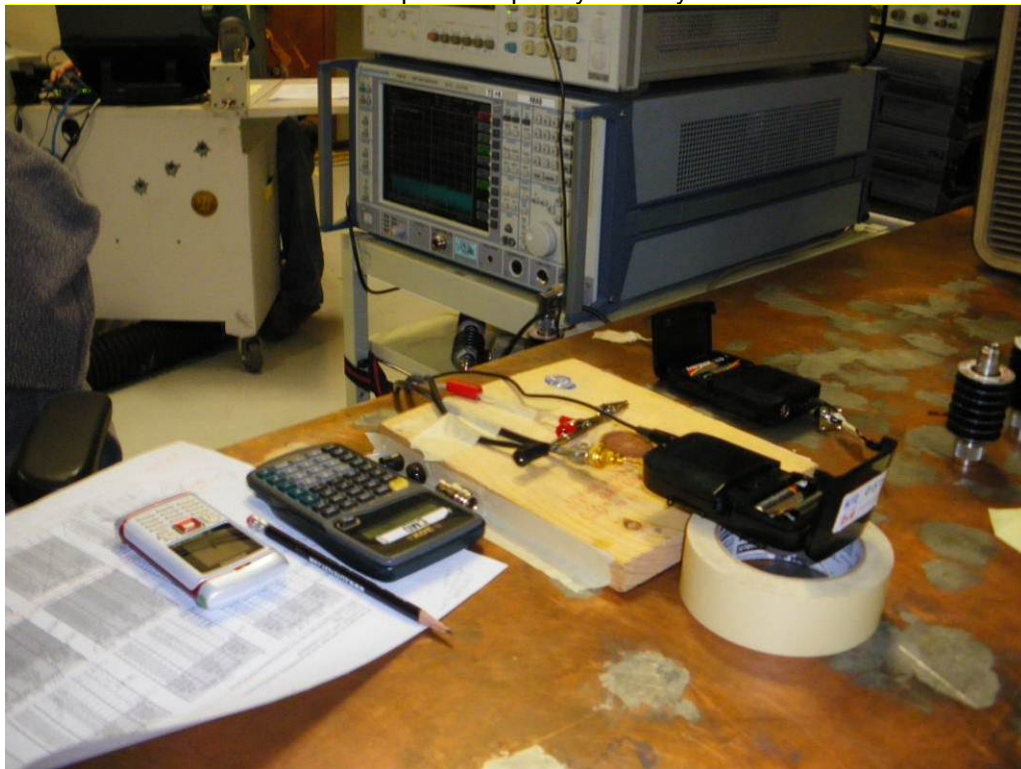
Test Setup for Occupied Bandwidth Test
