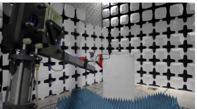
Figure 2: AXT200 Transmitter Test Setup
