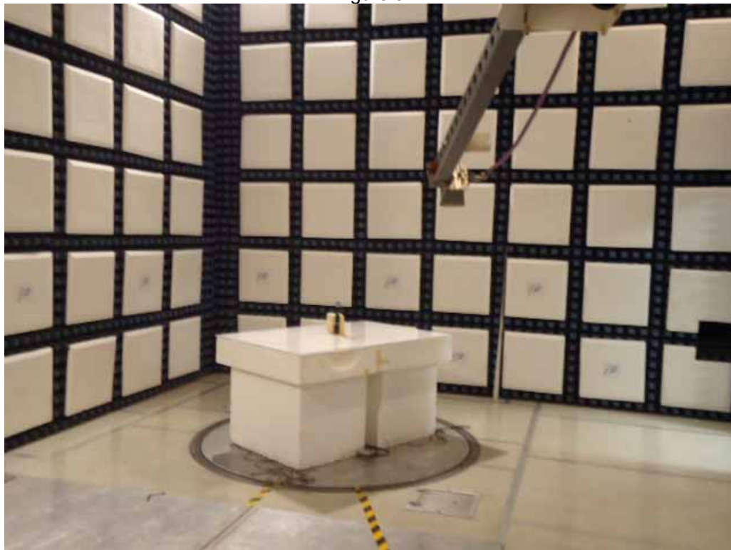
Test Setup for Radiated Emissions – 12GHz to 18GHz, Horizontal Polarization
