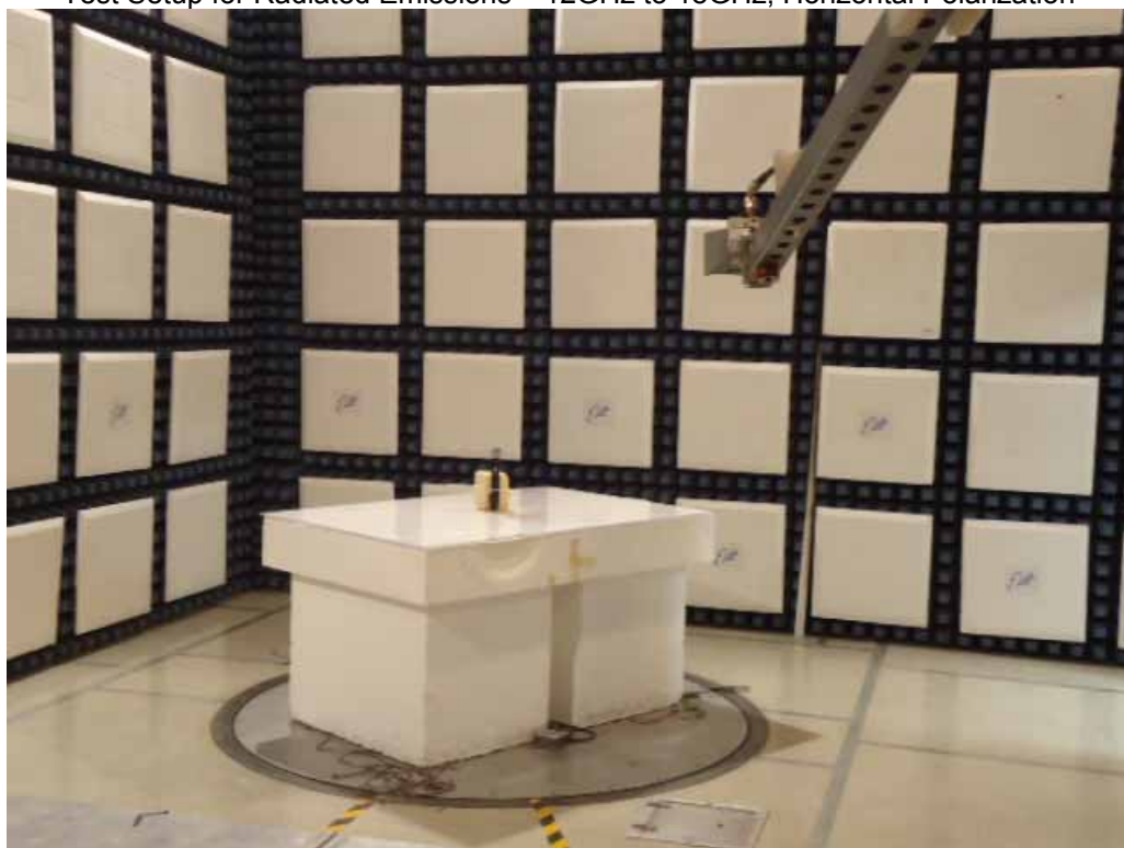
Test Setup for Radiated Emissions – 12GHz to 18GHz, Vertical Polarization
