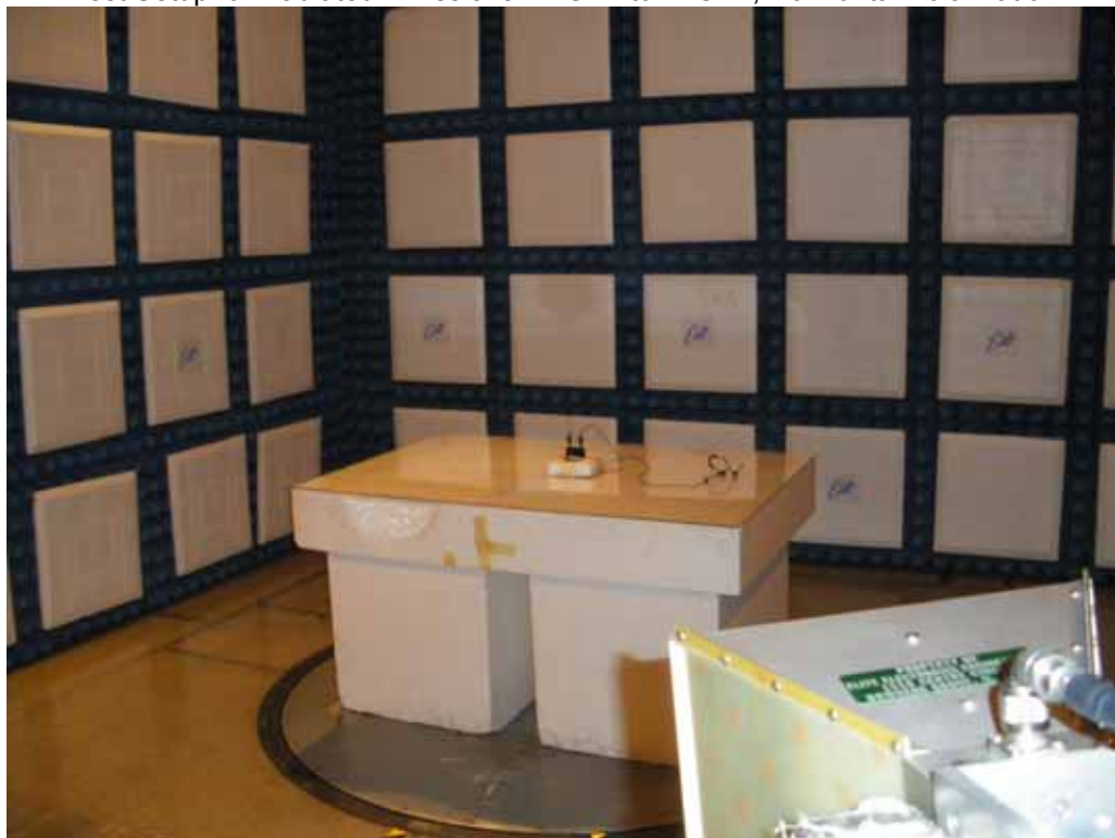
Test Setup for Radiated Emissions – 1GHz to 12GHz, Vertical Polarization
