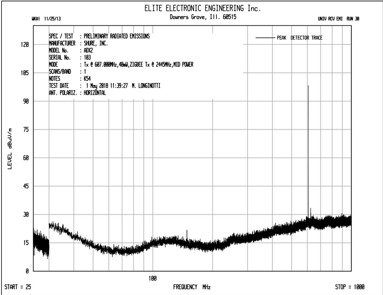
Plot shows emissions at 607.000MHz from UHF transmitter.
