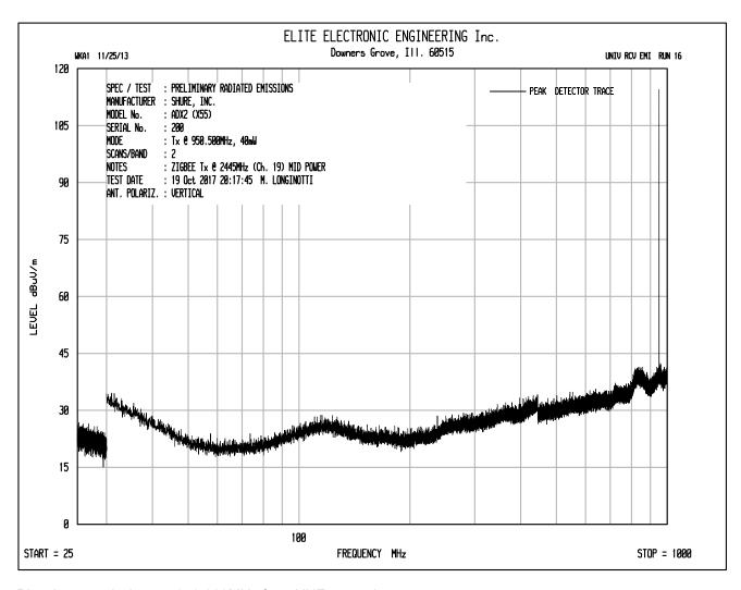
Plot shows emissions at 950.000MHz from UHF transmitter.
