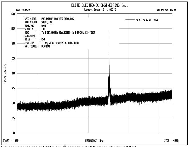
Plot shows emissions at 1214MHz (2<sup>nd</sup> harmonic of UHF transmitter of 607MHz).
