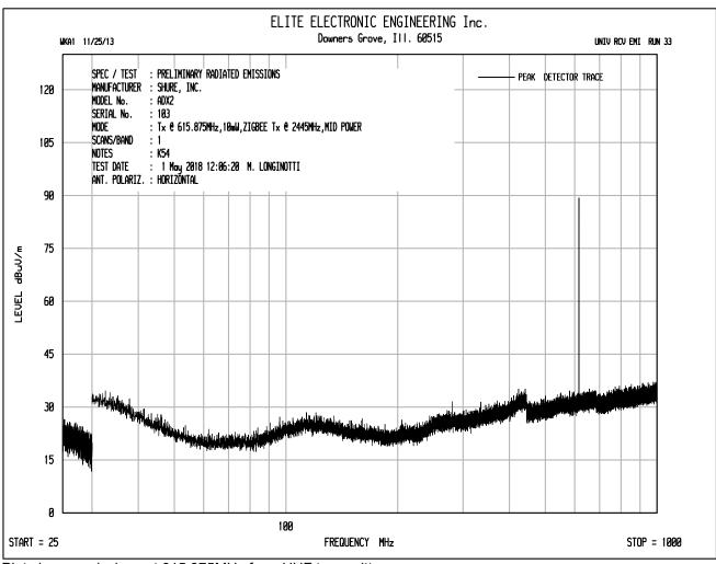
Plot shows emissions at 615.875MHz from UHF transmitter.
