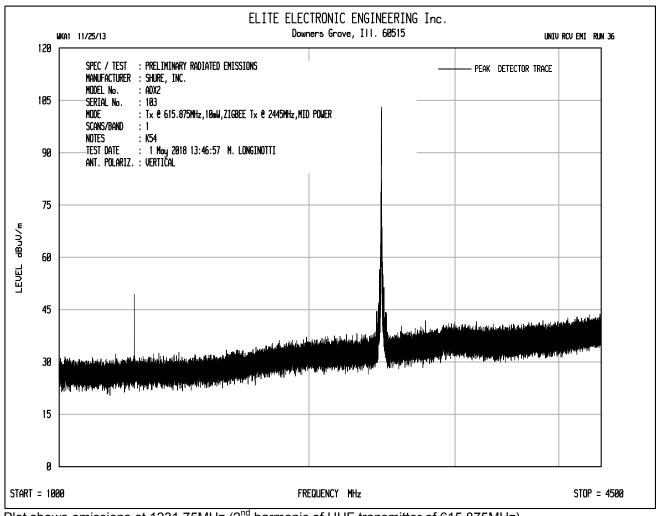
Plot shows emissions at 1231.75MHz (2<sup>nd</sup> harmonic of UHF transmitter of 615.875MHz). Plot shows emissions at 2445MHz from Zigbee transmitter.
