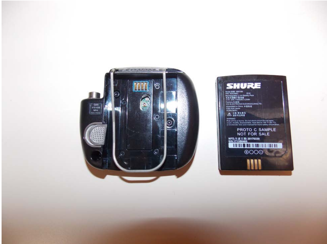
Back of Device with Li-Ion Battery
